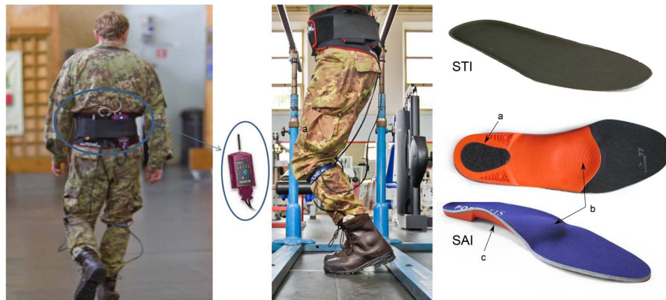
FIGURE 1. Left: Picture taken during the military training. The Pedar-x belt attached to the subject's back and Pedar-x box attached to the sensed insoles. The subject is wearing tested military boots. Right: The standard Insole and the shock-absorbing insole. Arrows point out differences among insoles (a: shock-absorbing heel pad; b: metatarsal support; c: elastic arch support).
